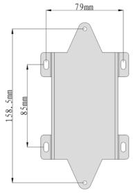
Figure 4: Mounting Bracket
