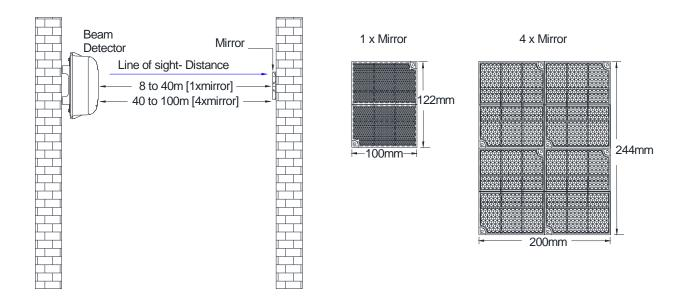
Figure 6: Mounting of Reflector Mirror
