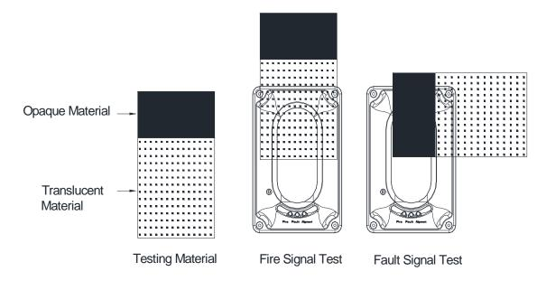
Figure 14: Testing Details
