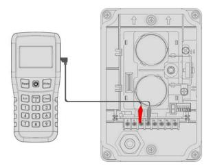
Figure 8: Programming connection Details
