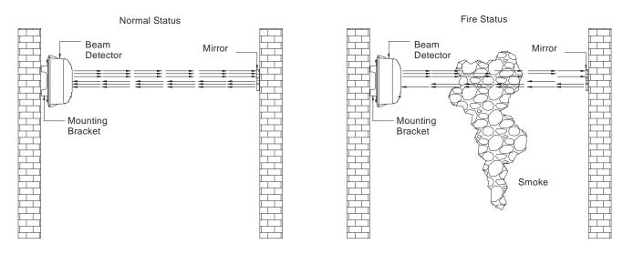
Figure 1: Beam detector principle
