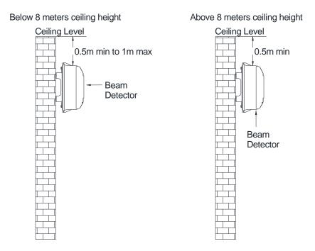
Figure 3: Installation Details
